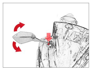
• Loosen the bolt slightly and adjust the holding pole to a preferred position so that you can have a good view of the rear.
