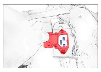
• To charge the bike, open the charging port lid and plug in the charger.
