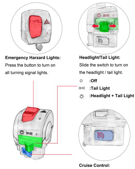
Press the button to activate the cruise control. To cancel the cruise function, press the button again or apply the brake.
