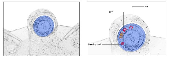
• The ignition is located at the front of the bike, centre of the handlebar.
