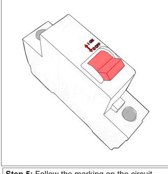
**Step 5:** Follow the marking on the circuit breaker, switch the circuit breaker off.
