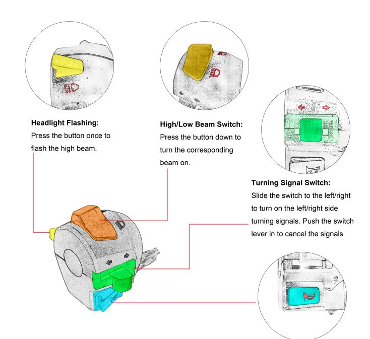
Horn Button: Press the button to sound the horn.
