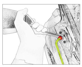
• Hold the mirror firmly in place and tightened the bolt with the allen key.
