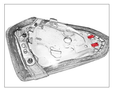
**Step 7:** When putting the seat back, make sure the teeth on the bottom of the seat (highlighted in red) are inserted into the holes.
